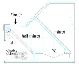
Fig. 3 Display box structure
